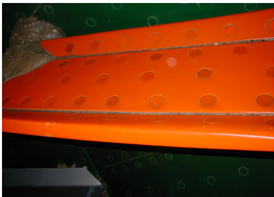
A Durex wrap-around blade liner on a Rex blade shows little wear after 2.5 years of mixing performance
