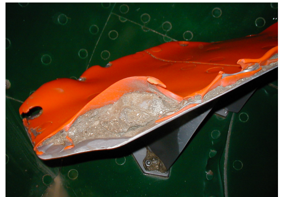
A traditional nonwrapping discharge blade liner is subject to considerable premature wear and peeling
